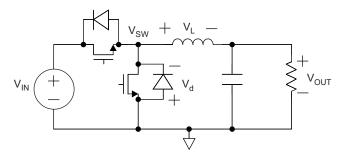
Figure 1. Synchronous Buck Converter
