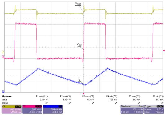
Figure 7. TPS62240 EVM, Poor Output Capacitor Placement
