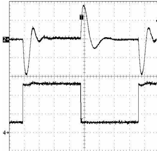
Figure 4. Undercompensated → R_C is Too Small
