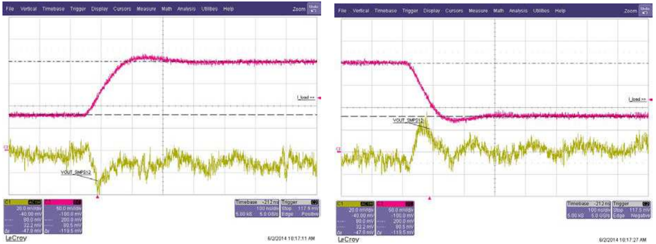
Figure 15. Dual-Phase Load-Step Response 5-V Input, 3.3-V Output, 194 \mu F, Hot
