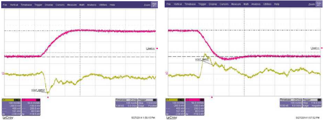
Figure 10. Single-Phase Load-Step Response 5-V Input, 3.3-V Output, 94 \mu F, Hot
