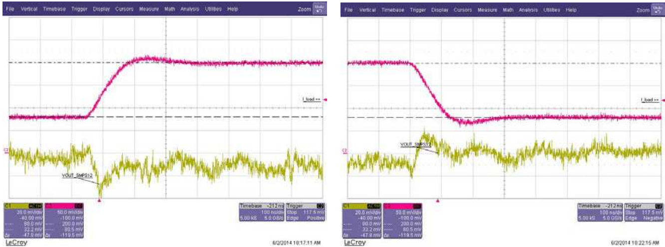
Figure 12. Dual-Phase Load-Step Response 3.3-V Input, 1.8-V Output, 194 \mu F, Hot
