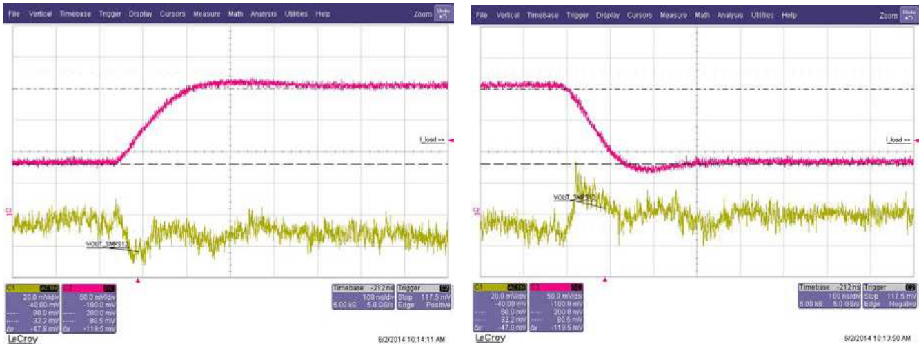
Figure 13. Dual-Phase Load-Step Response 5-V Input, 1.05-V Output, 194 \mu F, Hot
