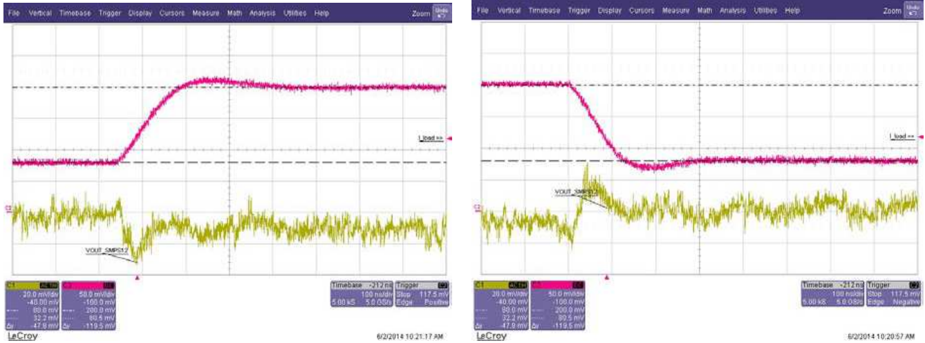
Figure 14. Dual-Phase Load-Step Response 5-V Input, 1.8-V Output, 194 \mu F, Hot
