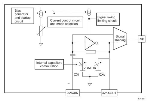
Figure 1. TPS659xx 32-kHz Internal Block Diagram
