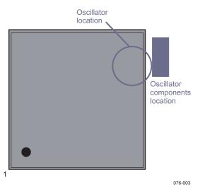
Figure 3. Best Placement for Crystal and Components
