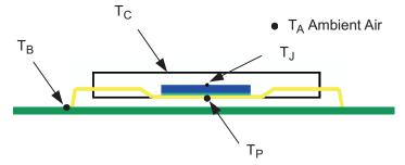
Figure 16. Thermal Resistance Diagram
