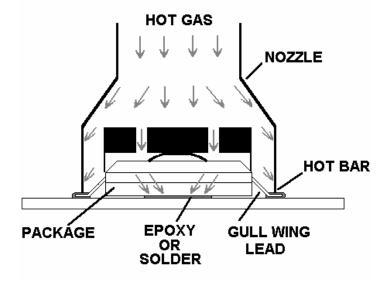
Figure 26. Nozzle Configuration
