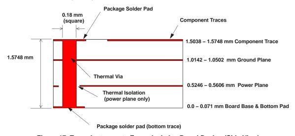
Figure 17. Texas Instruments Example Jedec Board Design (Side View)
