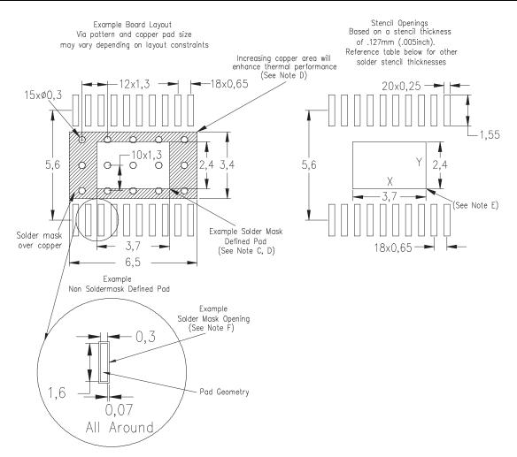
Figure 5. Package and PCB Land Configuration for a Multi-Layer PCB
