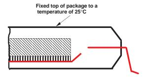
Figure 21. Standard Package  $\theta_{JC}$  Measurement
