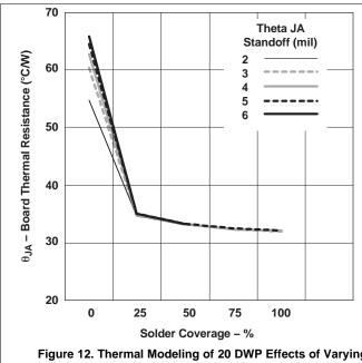
Figure 12. Thermal Modeling of 20 DWP Effects of Varying Solder Coverage and Standoff Height on  $\theta_{JA}$
