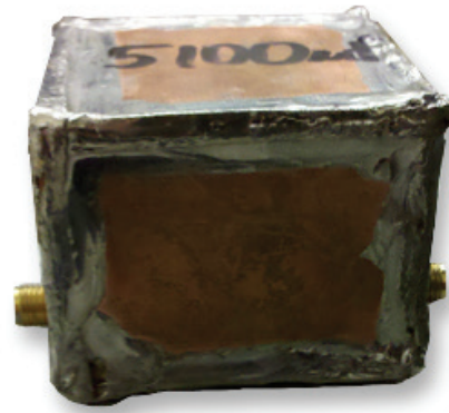
Figure 3. Our shielded 5100 \mu\text{F} AC-coupling cap which is used for making low noise measurements.
