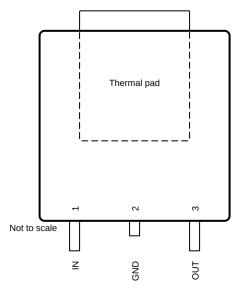
Figure 5-1. KVU Package, 3-Pin TO-252, Top View
