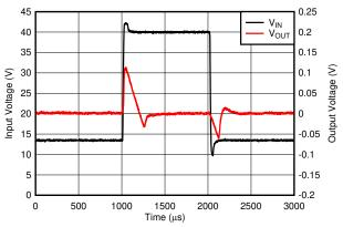
Line Transient Response (3-V/µs VIN Slew Rate)
