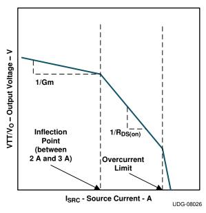
Figure 22. TPS7H3301-SP Impedance Characteristics
