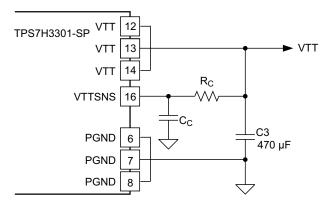
Figure 15. R-C Filter for VTTSNS
