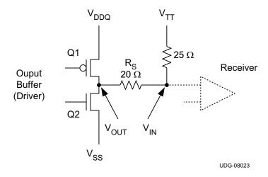
Figure 19. DDR Physical Signal System SSTL Signaling
