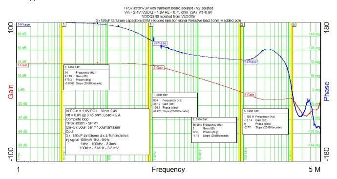
Figure 23. DDR2 2-A Load  $V_{IN} = 2.4 \text{ V}$ , VTT/ $V_{O} = 0.9 \text{ V}$
