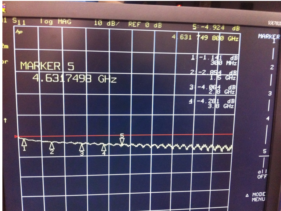
Figure 10. Cable Losses versus Frequency
