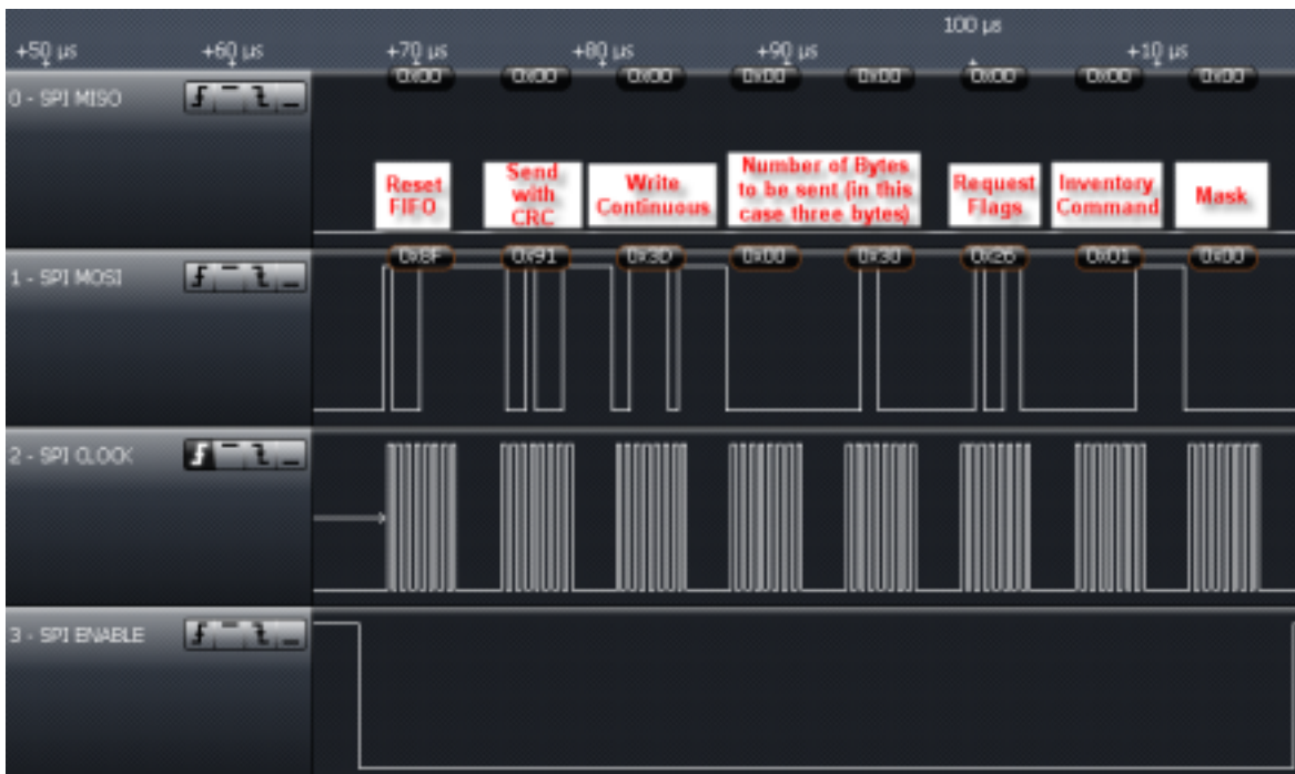
Figure 6-22. Inventory Command Sent From MCU to TRF7964A
