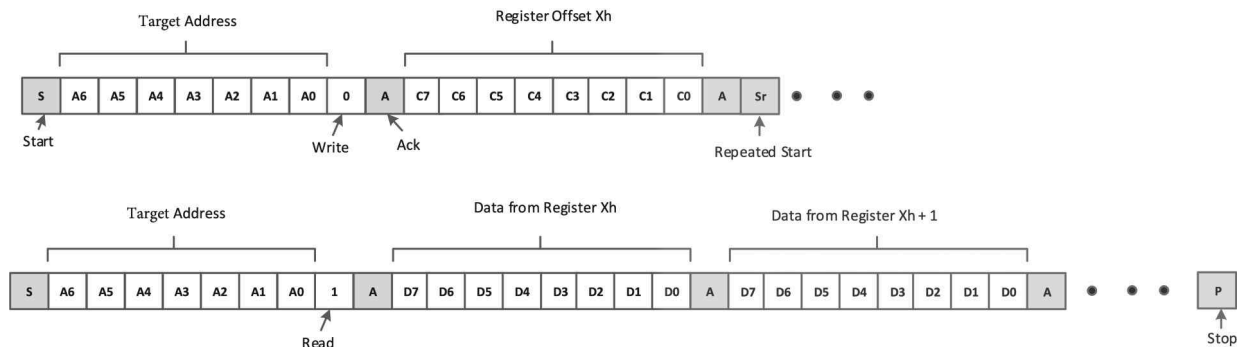
Figure 8-8. I 2 C Read with Repeated Start
