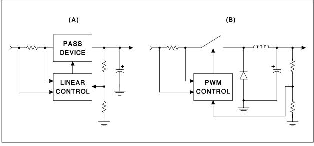
Figure 1. Basic elements of a A.) Linear and B.) Switching Regulator.
