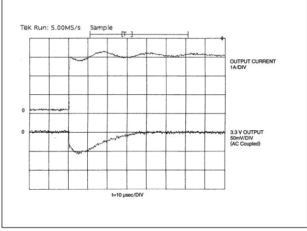
Figure 5: Transient response of the regulator illustrated in Figure 2 with a time base of 10 µsec.
