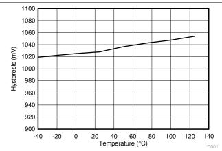
Figure 6-18. 8-V UVLO Threshold vs. Temperature
