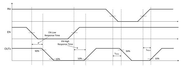
Figure 7-3. Enable Pin Timing
