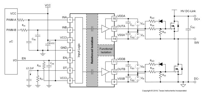
Figure 9-1. Typical Application Schematic with Dual Power Supplies
