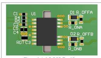
Figure 9-4. 3-D PCB Top View
