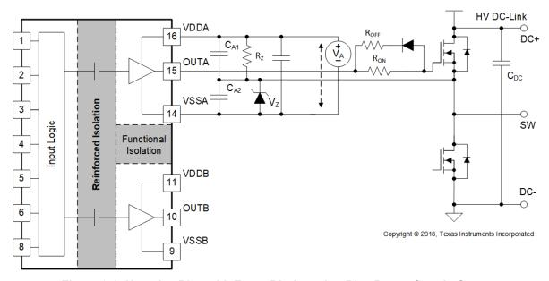
Figure 9-2. Negative Bias with Zener Diode on Iso-Bias Power Supply Output
