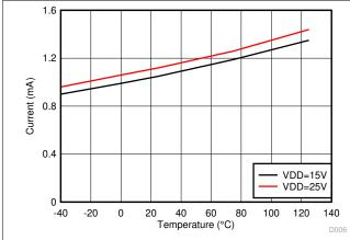
Figure 6-8. Per Channel (I<sub>VDDA/B</sub>) Quiescent Supply Current vs Temperature (No Load, Input Low, No Switching)
