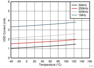
Figure 6-7. Per Channel (I<sub>VDDA/B</sub>) Supply Current Vs. Temperature (VDD=15V, No Load, Different Switching Frequencies)
