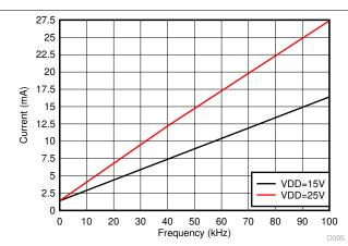
Figure 6-6. Per Channel Current Consumption (I<sub>VDDA/B</sub>) vs. Frequency (10-nF Load, VDD = 15 V or 25 V)
