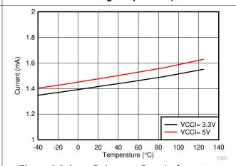
Figure 6-9. I<sub>VCCI</sub> Quiescent Supply Current vs Temperature (No Load, Input Low, No Switching)
