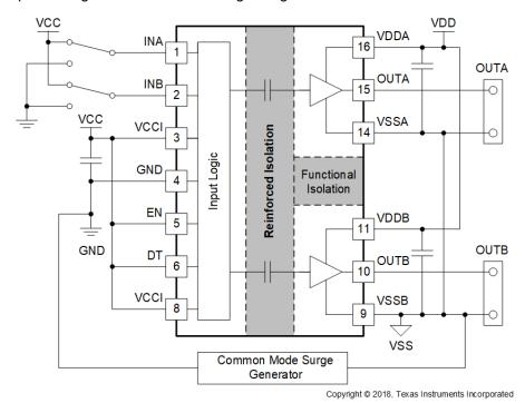
Figure 7-7. Simplified CMTI Testing Setup
