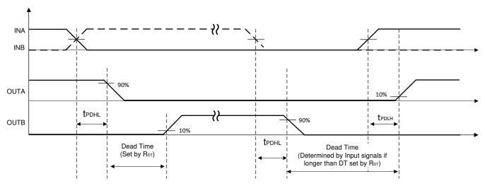
Figure 7-4. Dead-Time Switching Parameters
