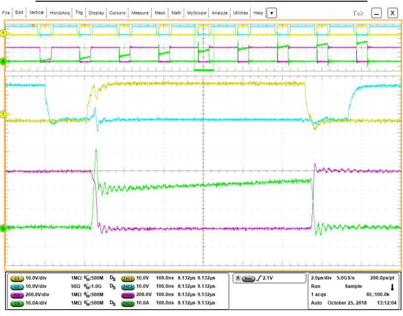
Figure 9-6. SiC MOSFET Switching Waveforms
