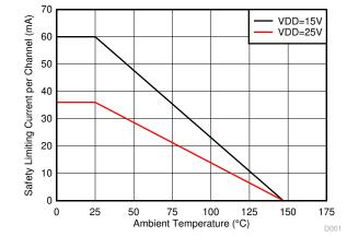
Figure 6-2. Thermal Derating Curve for Safety-Related Limiting Current (Current in Each Channel with Both Channels Running Simultaneously)
