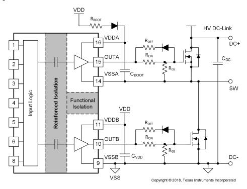
Figure 9-3. Bootstrap Power Supply for the High Side Device
