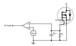
Figure 3. SenseFET Current Sensing Scheme
