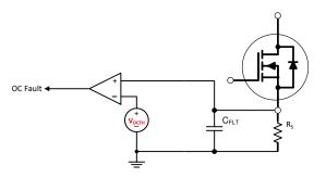
Figure 2. Shunt Resistor Current Sensing Scheme
