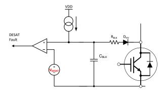
Figure 1. Desaturation Detection Circuit
