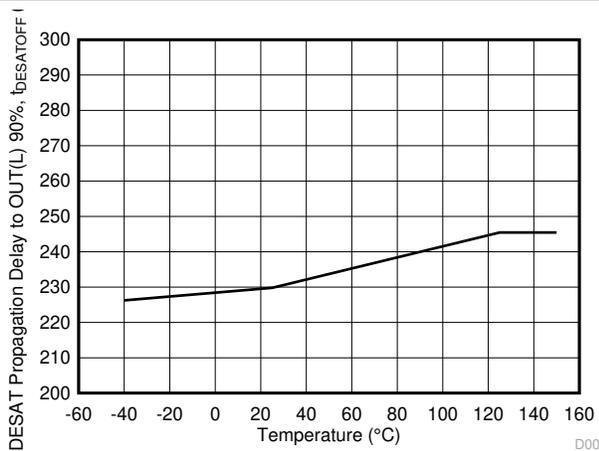
**Figure 6-25. t<sub>DESATOFF</sub> DESAT Propagation Delay to OUT(L) 90% vs. Temperature**
