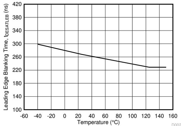
**Figure 6-24. t<sub>DESATLEB</sub> DESAT Leading Edge Blanking Time vs. Temperature**
