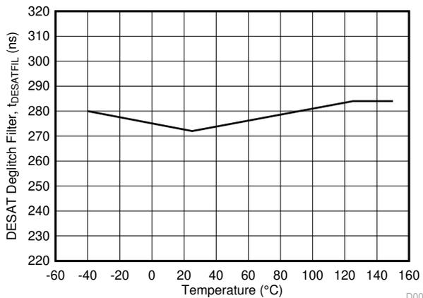
**Figure 6-27. t<sub>DESATFIL</sub> DESAT Deglitch Filter vs. Temperature**
