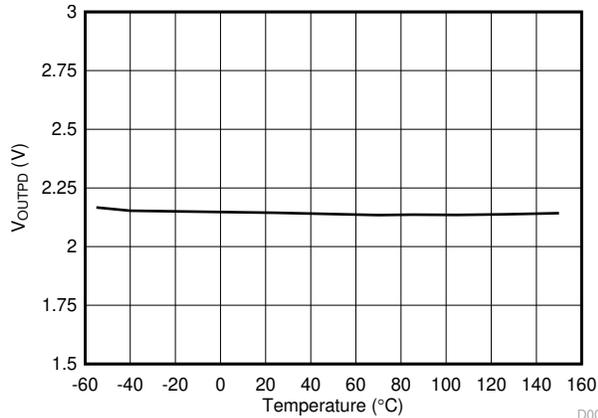
**Figure 6-17. V<sub>OUTPD</sub> Output Active Pulldown Voltage vs. Temperature**
