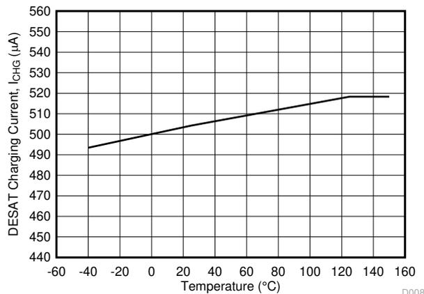
**Figure 6-28. I<sub>CHG</sub> DESAT Charging Current vs. Temperature**
