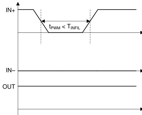
Figure 7-4. IN+ OFF Deglitch Filter
