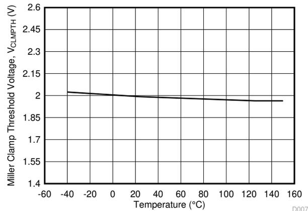
**Figure 6-20. V<sub>CLMPH</sub> Miller Clamp Threshold Voltage vs. Temperature**
