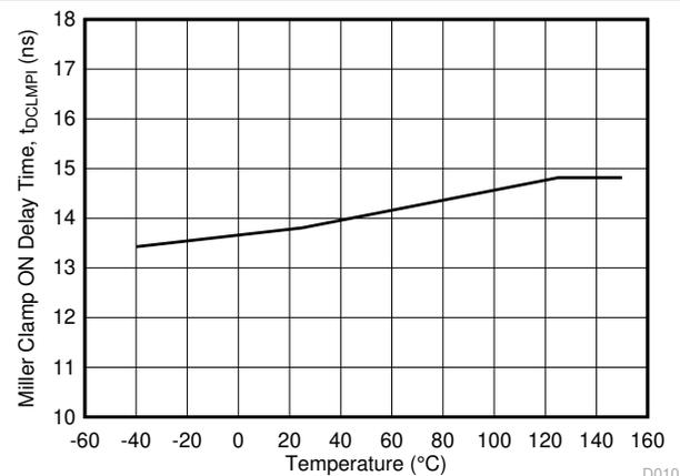
**Figure 6-22. t<sub>DCLMPI</sub> Miller Clamp ON Delay Time vs. Temperature**
