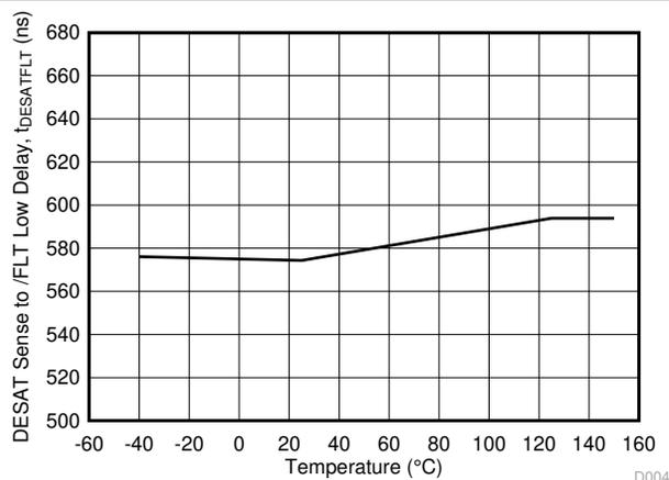
**Figure 6-26. t<sub>DESATFLT</sub> DESAT Sense to /FLT Low Delay Time vs. Temperature**
