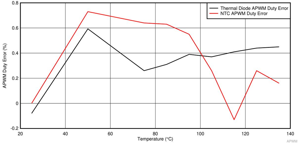
Figure 9-11. APWM Duty Error with Single-Point Calibration
