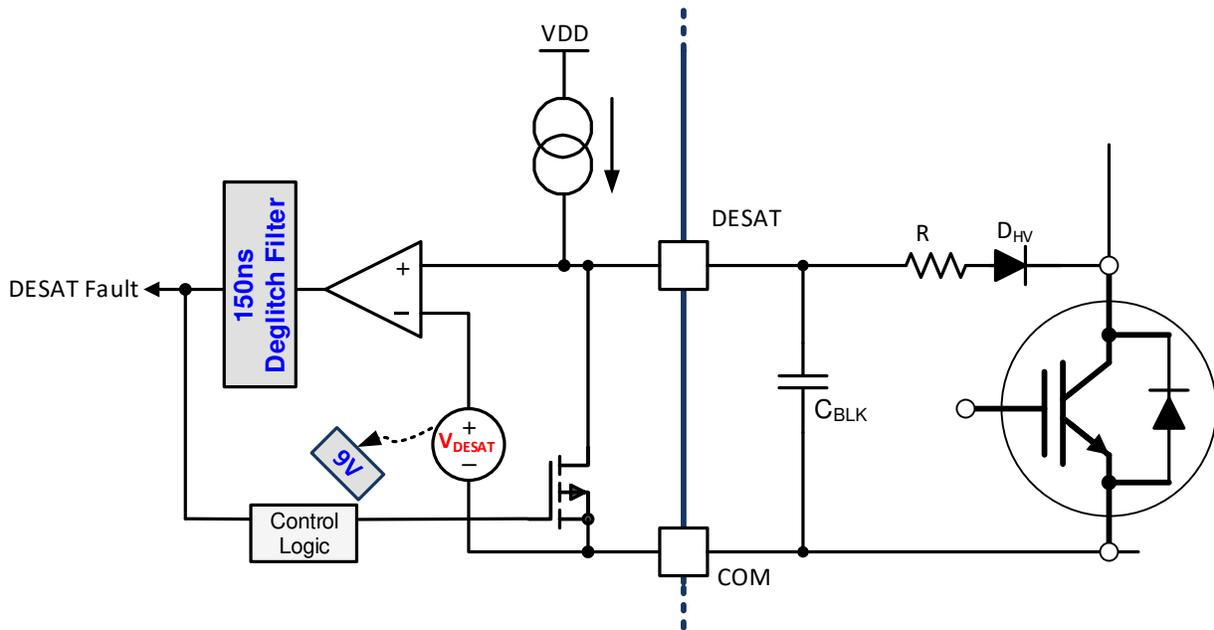
**Figure 8-5. DESAT Protection**
