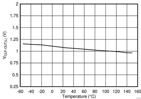
**Figure 6-19. V<sub>CLP-OUT(L)</sub> Short Circuit Clamping Voltage vs. Temperature**
