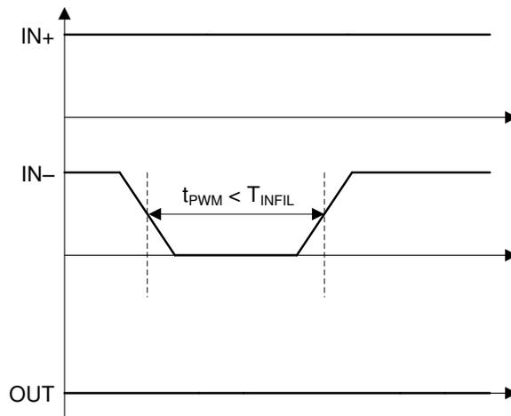
Figure 7-6. IN- OFF Deglitch Filter
