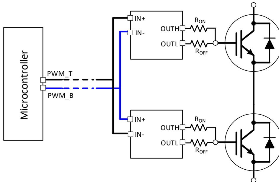
**Figure 9-2. PWM Interlock for a Half Bridge**
