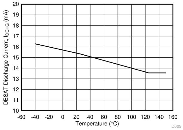
**Figure 6-29.  $I_{DCHG}$  DESAT Discharge Current vs. Temperature**
