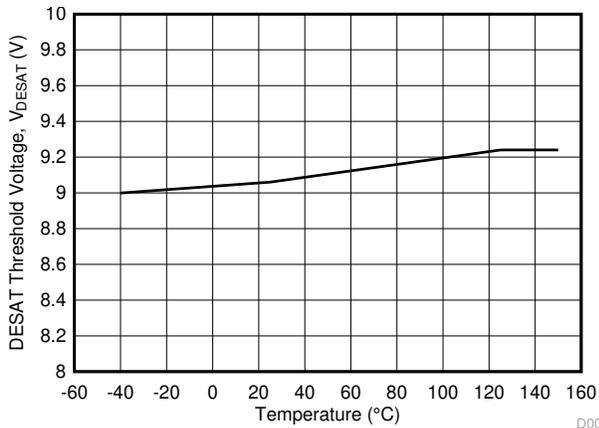
**Figure 6-23. V<sub>DESAT</sub> DESAT Threshold Voltage vs. Temperature**
