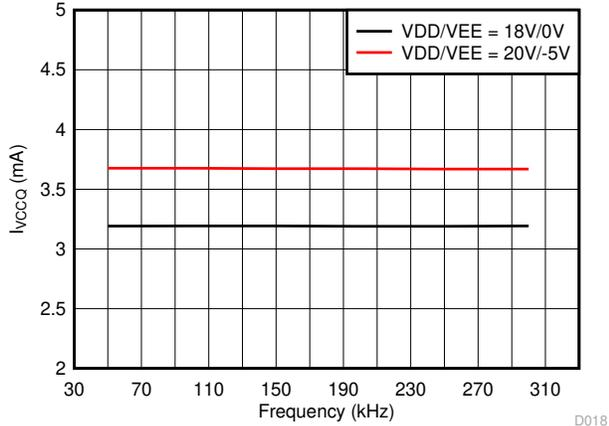
**Figure 6-7.  $I_{VCCQ}$  Supply Current vs. Input Frequency**
