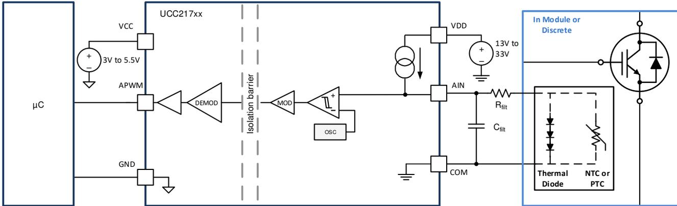
**Figure 9-7. Thermal Diode or Thermistor Temperature Sensing Configuration**
