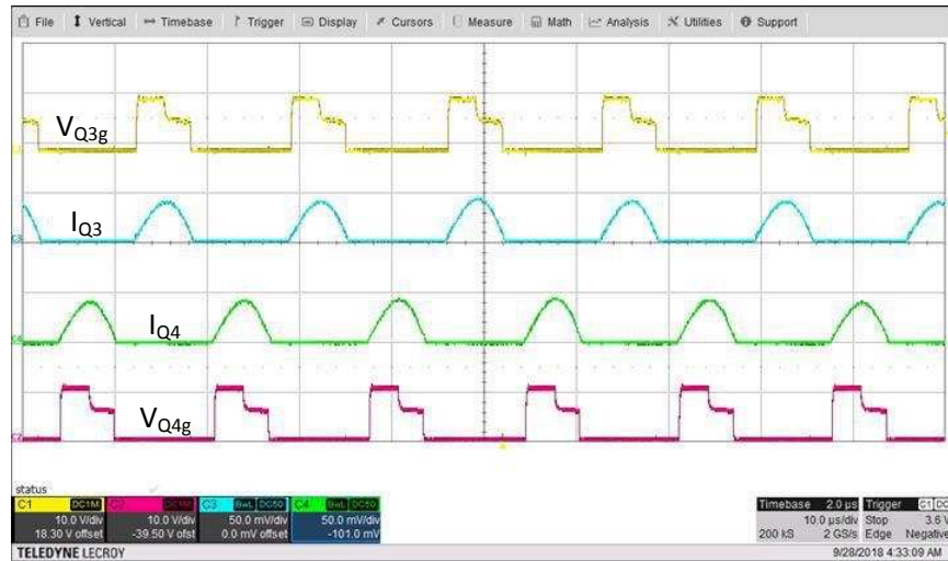
Figure 3. LLC ZVS Oscilloscope Waveforms
