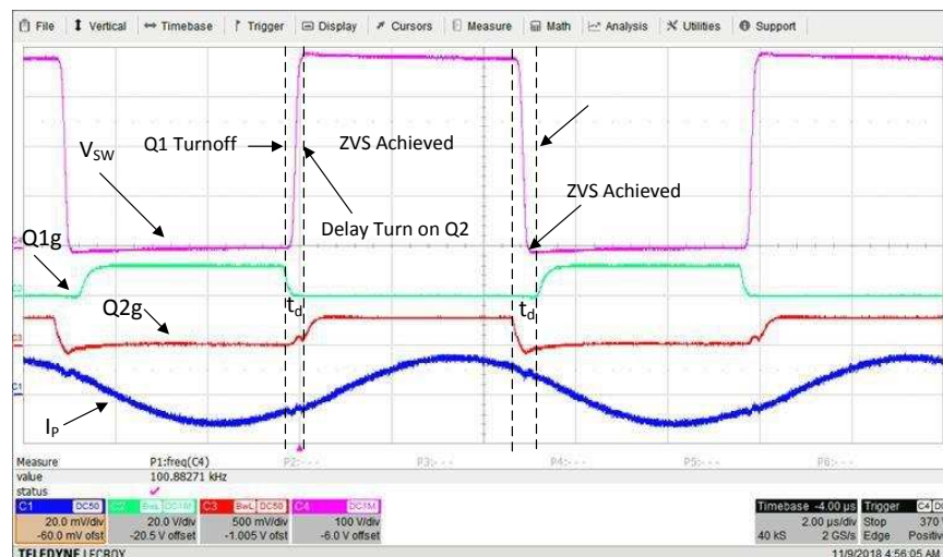
Figure 2. LLC ZVS Oscilloscope Waveforms
