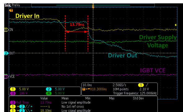
Figure 8-3. UCC27624-Q1 Used to Drive IGBT in the Boost Converter
