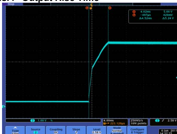
Full load rise time at 90V input CH2:1V/div
