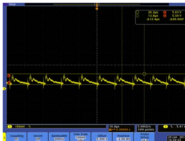
Figure 18. Full load output voltage Ripple in 115Vac and 230Vac
