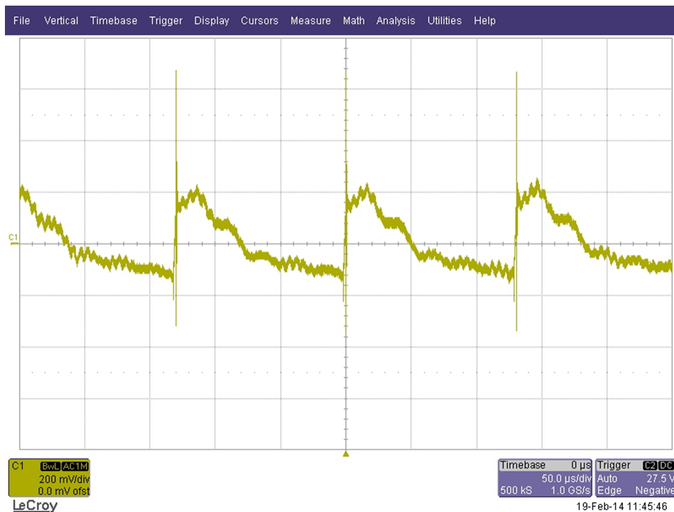
Figure 20. Vout Ripple at Vin = 275 VAC, Full Load
