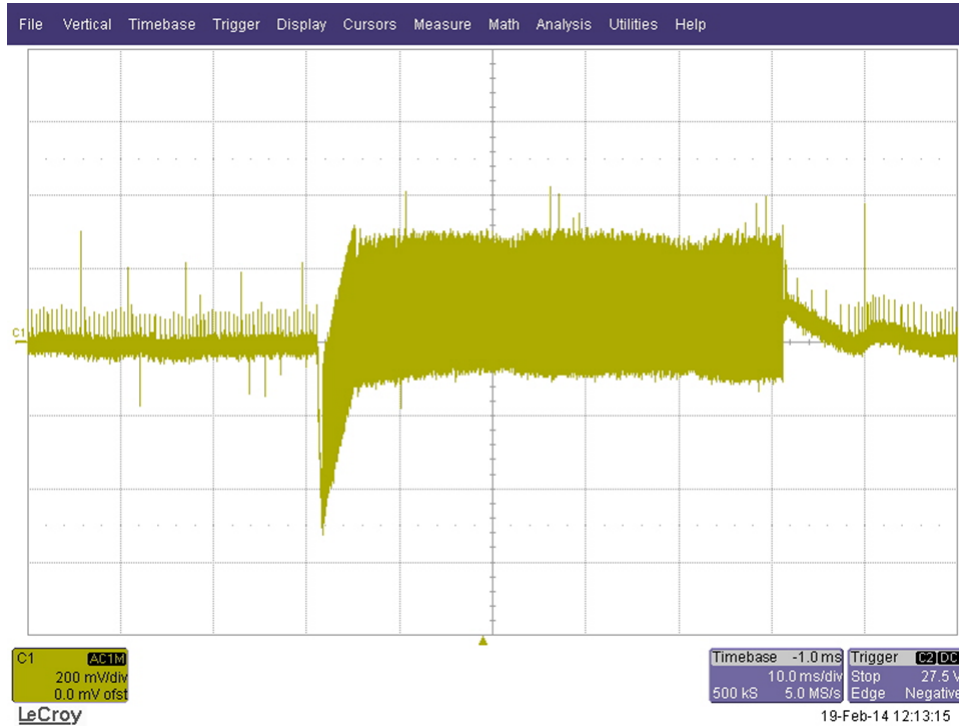
Figure 23. Vout Waveform at Vin = 230 VAC, Load Transient from 2 mA to 200 mA
