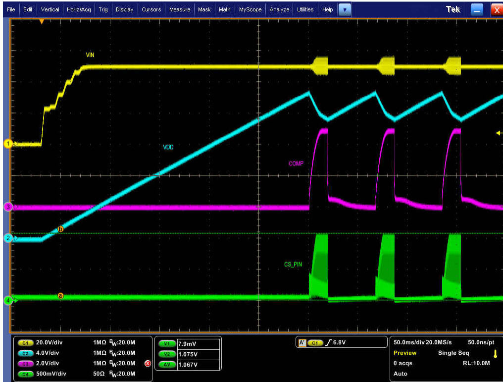
Figure 5-27. 50 VIN, Startup with output shorted to ground
