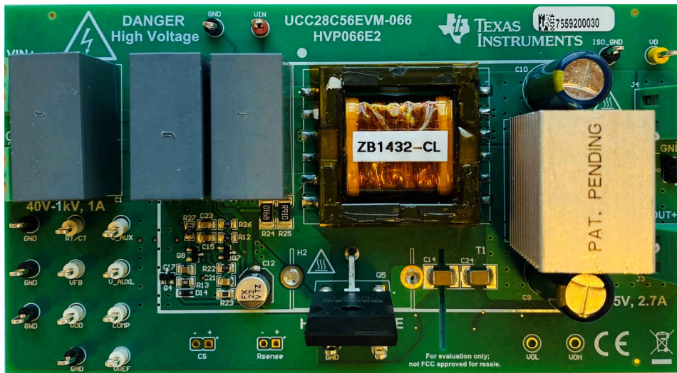
Figure 2-1. UCC28C56EVM-066, HVP066E2, Top View
