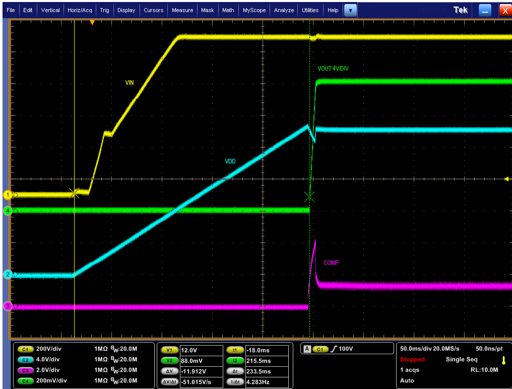
Figure 5-9. Start-Up 3: VIN = 1000 V, Load = 0.25 A
