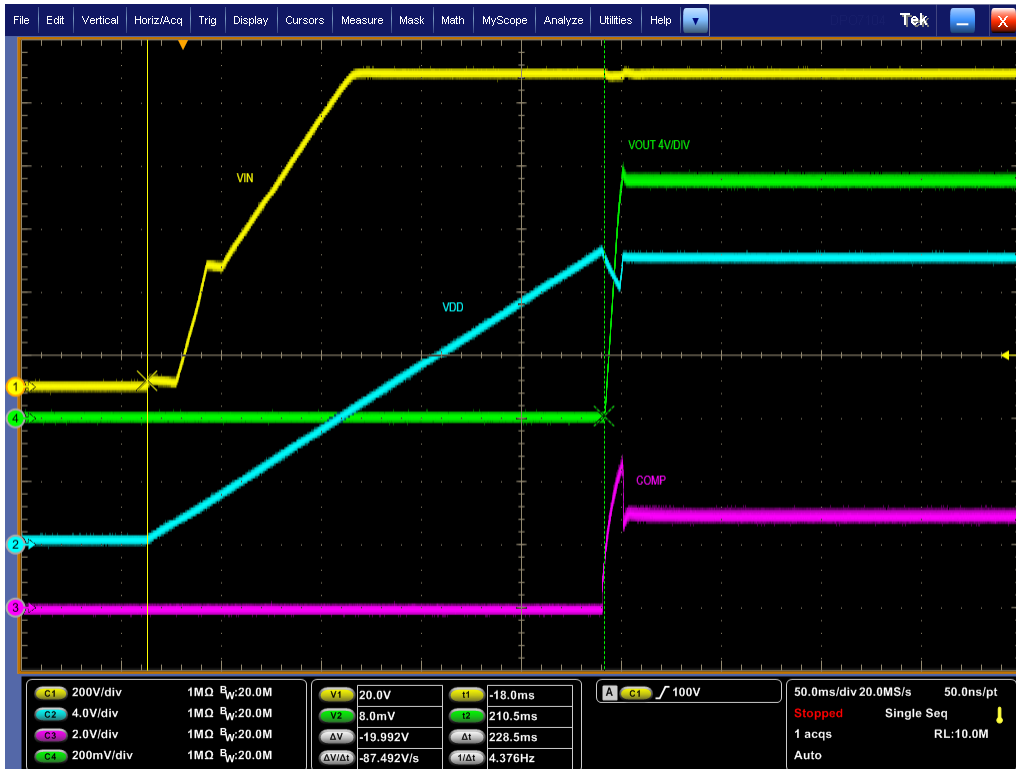
Figure 5-10. Start-Up 4: VIN = 1000 V, Load = 2.7 A
