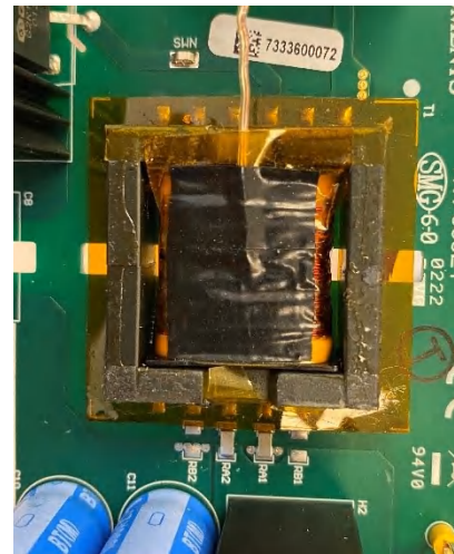
Figure 5-37. Black tape for thermal camera
