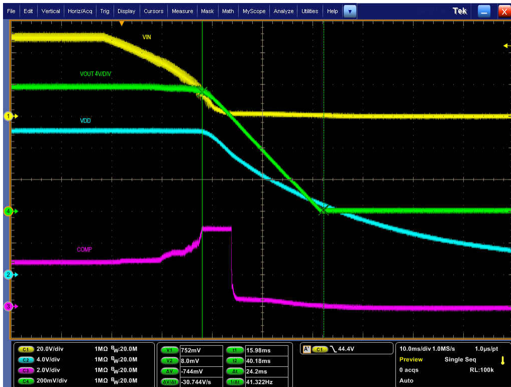
Figure 5-12. Shutdown, VIN Removal: VIN = 50 V, Load = 1.3 A
