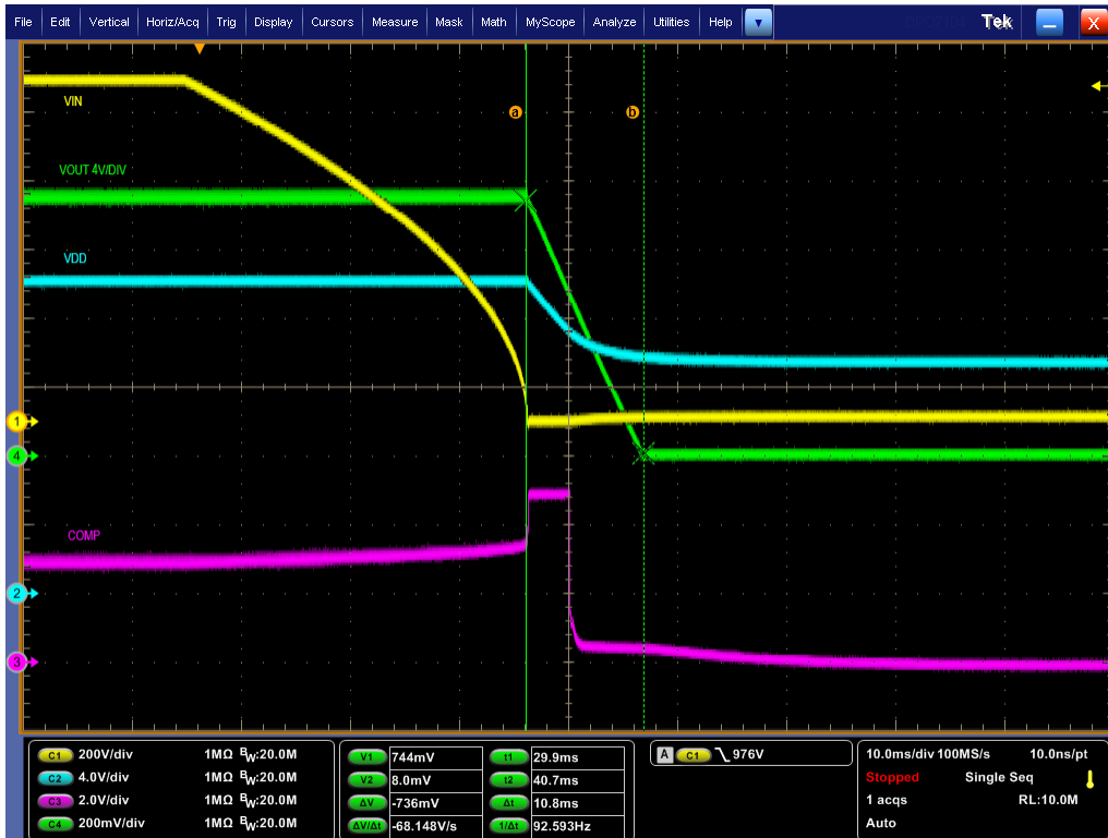
Figure 5-14. Shutdown, VIN Removal: VIN = 1000 V, Load = 2.7 A
