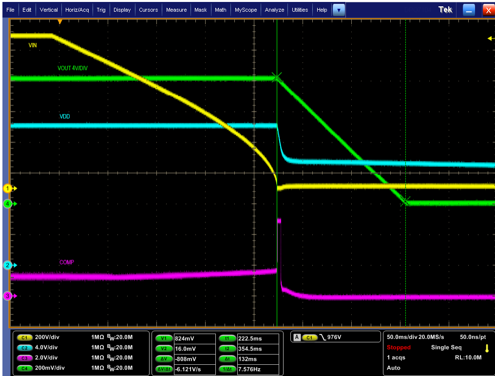
Figure 5-13. Shutdown, VIN Removal: VIN = 1000 V, Load = 0.25 A
