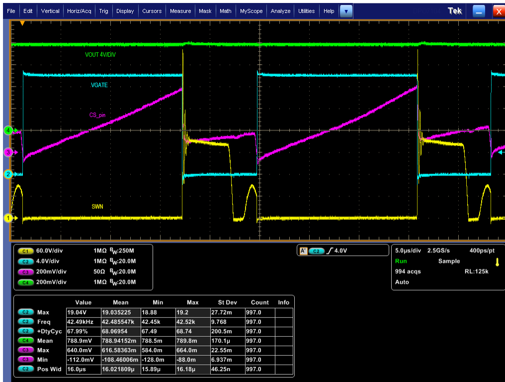
Figure 5-20. Steady State: VIN = 50 V, Load = 1.3 A
